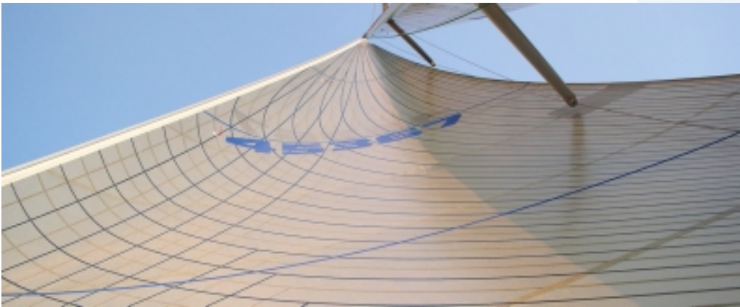
PROPER SAIL SHAPE OF GENOA IN 12 KNOTS TRUE WIND
